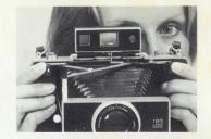
**TWO** is for shooting. Press the No. 2 button slowly, being careful not to move the camera. With slow shutter speeds, hold the button down and keep the camera still until you hear the second click as the shutter closes.
