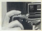
3. RESET: Immediately after taking a picture, press the No. 3 button down firmly all the way; then let it up again. This resets the shutter so you'll be ready for the next picture.
