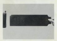
Pull the safety cover all the way out of the camera without stopping. Pull straight so you won't rip it. Discard the safety cover.
