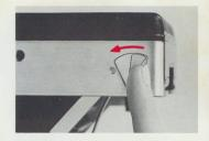
Open the back all the way. Note the steel rollers. They must be kept clean as shown on page 26.
