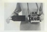
The picture develops outside the camera. While it's developing, hold the tab by the yellow tip, or lay the picture assembly down flat; don't touch or bend the picture assembly or lift off the white paper (A). Outdoors, don't let the picture assembly flap in the breeze. Develop the picture for the full time recommended in the instruction sheet packed with the film.
