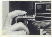
THREE is for resetting. After taking a picture, always push down the No. 3 button firmly; then let it come up again. This resets the shutter for the next picture. If you don't reset the No. 3 button, nothing will happen when you press the No. 2 button for your next picture.
